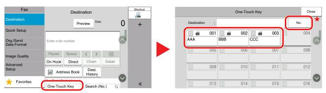
The [No.] key has the same function as [Search (No.)] displayed on the touch panel. Use to directly enter a number with the numeric keys, such as specifying a transmission address using a one-touch key number, or calling up a stored program using the program number. For information on one-touch key numbers, refer to the following:
