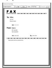
To display a different template, use the drop-down menu at the top of the dialog box or click on the  $[\blacktriangleleft]$  or  $[\blacktriangleright]$  button. The template display magnification can also be changed within the range of 25 to 250% from the drop-down menu.
